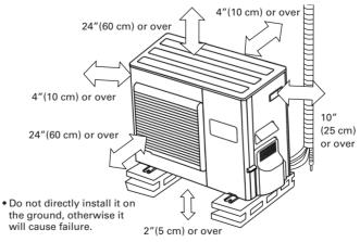
To obtain better operation efficiency, when the outdoor unit is installed, be sure to open the front and left side.
