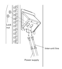
Keep the earth wire longer than the other wires
